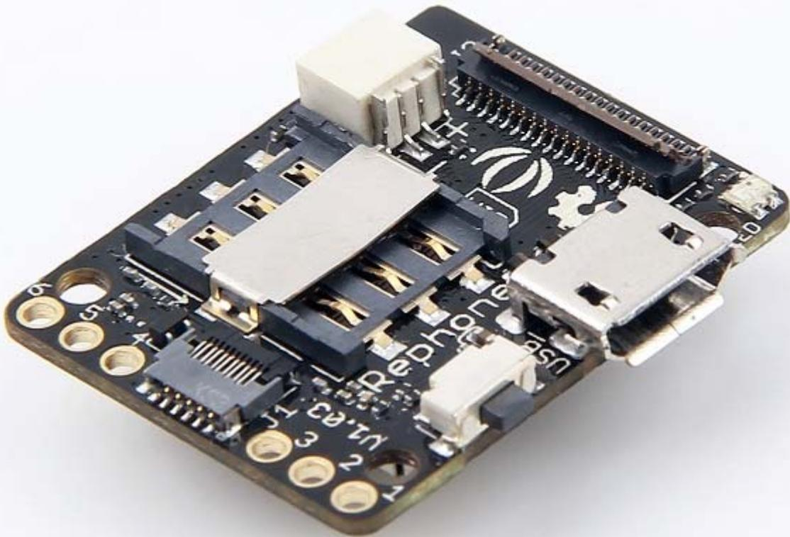
Whether making and receiving telephone calls over a radio link using external speakers and microphone or exchanging data in short distances with Bluetooth, you can do it with Xadow GSM+BLE.
