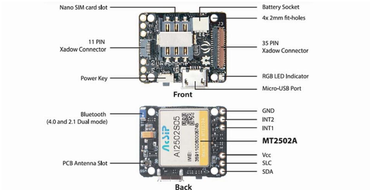
The image below illustrates the Pin Definitions of 11 Pin Xadow Connector, Solder-able Breakout Pins and the 35 Pin Xadow Connector in a sequence from **Left to Right**.
