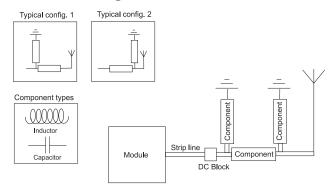
The matching network has to be individually designed using one, two or three components.
