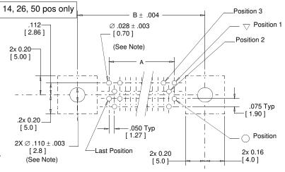
Note: Plated through holes for .062" board thickness.
