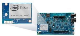
This kit includes an Arduino Breakout, which essentially gives your Edison the ability to interface with Arduino shields or any board with the Arduino footprint.
