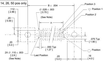
Note: Plated through holes for .062  $\!\!^{\prime\prime}$  board thickness.
