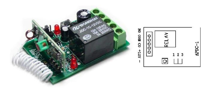
A wireless relay is a codec-adaptive RF receiver with single channel relay. It helps easily
