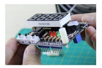
From below, secure the standoffs to the board, by screwing a nut onto each one.
