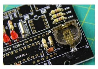
Now let's move on to the sockets. Search for the half-moon shape on the board. This is the directional indicator for the IC Sockets. It is very important that the orientation of the IC socket is correct. After soldering the 4 LEDs and 2 sensors, the board should look like this:
