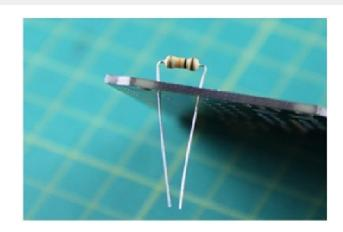
Bend its leads out so you can hold it in place when soldering.
