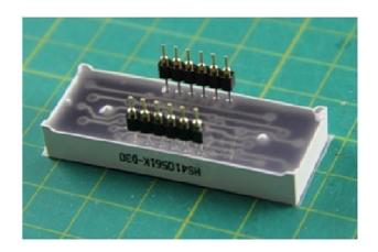
Now insert the 7-segmentdisplay onto the board. Match up the printed side of the 7-segment display with the solid circles on the board.
