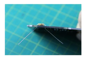
Flip over the board, and we can solder one lead at a time. Make sure the tip of your soldering iron is shiny. If not, melt some solder on it and quickly wipe it on the wet sponge.
