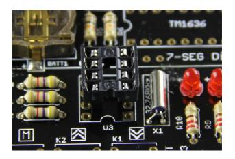
There are eight legs for the U3 socket. Place your finger on the socket to keep it in place when you flip over the board. Quickly spread some solder onto one of the legs.
