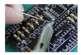
Now flip over the board and solder the crystal's two leads.
