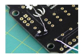
We don't need the excess lead (the wire sticking out of the board). So when you're done, use the flush cutter to cut the excess and make it flush with the board. Be very careful when doing this as the lead will fly off after cutting it. Turn the board to one side to prevent the lead from inadvertently injuring you. It is highly recommended that you wear eye protection during this step.
