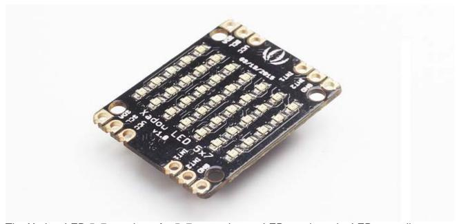
The Xadow LED 5x7 consists of a 5x7 monochrome LED matrix and a LED controller. You can sending command to the LED controller through I2C interface (address 0x21) to display numbers, letters or even pixel images. This could come handy sometime in your project.
