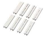
Zack marker strip, Strip, white, Labeled, Printed horizontally: Consecutive numbers 1 - 9, Mounting type: Snap into tall marker groove, For terminal block width: 5.2 mm, Lettering field: 5.15 x 10.5 mm
