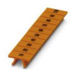
Marker for terminal blocks, Strip, orange, labeled, printed horizontally: Sets of ten 10 - 100, mounting type: snap into tall marker groove, for terminal block width: 5.2 mm, lettering field size:  $10.5 \times 5.15 \text{ mm}$
