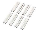
Zack marker strip, Strip, white, Labeled, Can be labeled with: Plotter, Horizontal: L1, L2, L3, N, PE, L1, L2, L3, N, PE, Mounting type: Snap into tall marker groove, For terminal block width: 5.2 mm, Lettering field: 5.15 x 10.5 mm
