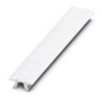
Zack marker strip, Strip, white, Labeled, Can be labeled with: Plotter, Printed horizontally: U, V, W, N, GND, U, V, W, N, GND, Mounting type: Snap into tall marker groove, For terminal block width: 6.2 mm, Lettering field:  $6.15 \times 10.5$  mm
