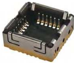
8.50 by 8.50mm, SMT, Through-board, 24 circuits Side Contact, 4.20mm height (Series 47337)
