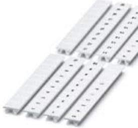
Zack marker strip, Strip, white, Labeled, Printed horizontally: Consecutive numbers 1 - 9, Mounting type: Snap into tall marker groove, For terminal block width: 8.2 mm, Lettering field: 10.5 x 8.15 mm
