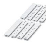
Zack marker strip, Strip, white, Unlabeled, Can be labeled with: Plotter, Mounting type: Snap into tall marker groove, For terminal block width: 7.62 mm, Lettering field: 10.5 x 7.5 mm
