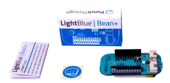
It is an Arduino-compatible board that you program wirelessly using Bluetooth Low Energy. With Bean+, you can program wirelessly from any of your devices. Bean+ also comes with a built-in accelerometer, temperature sensor and RGB LED.
