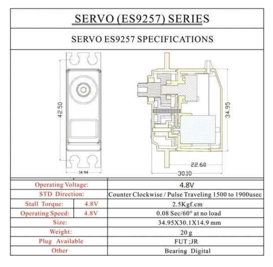
Note: This servo is recommended to use at 4.8V. (damage under higher voltage is not covered by warranty)
