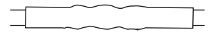
3. Heat crimped device with Master heat tool until tubing recovers and adhesive melts and flows.
