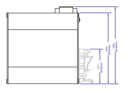
NOTE: These drawings reference the 108TX. Secure online The 108TX-HV dimensions are identical
