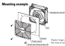
Plastic finger guards are placed on both the intake and exhaust sides of the fan. No nuts or screws for use in attachment included.
