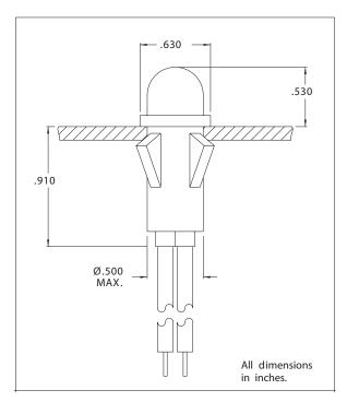
Mounting: Will snap-fit into Ø.500/.505 hole in panels .020/.100 thick. Push-on speednut SN0461 also available.
