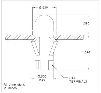
Solid-state indicator lights complete with built-in current-limiting resistor and rectifier diode.
