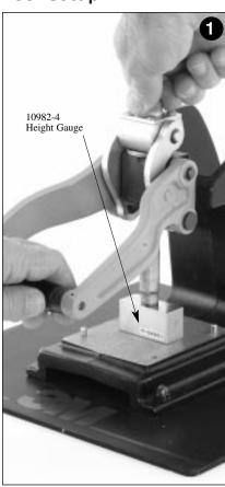
Place the 10982-4 height gauge on the base plate of the press (locator plate removed). Bring the handle down fully and adjust the shaft to touch the gauge. Raise the handle, remove the gauge then turn the adjustment screw one quarter turn (90 degrees) clockwise.
