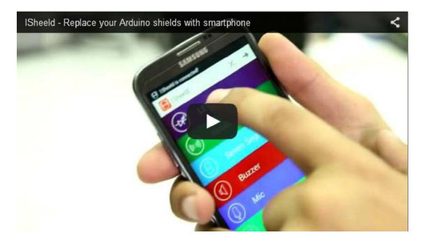
1Sheeld is a new easily configured shield for Arduino. It is connected to a mobile app that allow the usage of all of Android smartphones' capabilities such as LCD Screen, Gyroscope, Switches, LEDs, Accelerometer, Magnetometer, GSM, Wi-Fi, GPS ...etc. into your Arduino sketch.
