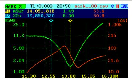
The *«Info»* option displays detailed information of the readings at the marker position, including the difference in frequency between both markers. One possible use of this feature is determining the VSWR bandwidth of an antenna.
