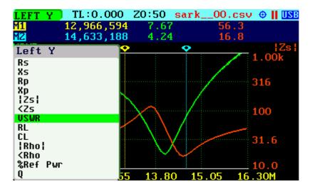
(ii) Use Navigator B when either the **«LEFT Y»** or **«RIGHT Y»** option is highlighted. Options are selected sequentially.
