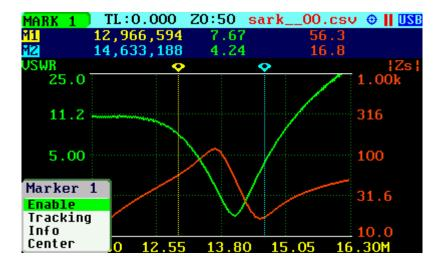
The automatic tracking feature makes positioning of the markers easier, thus helping the user to speed up measurements.
