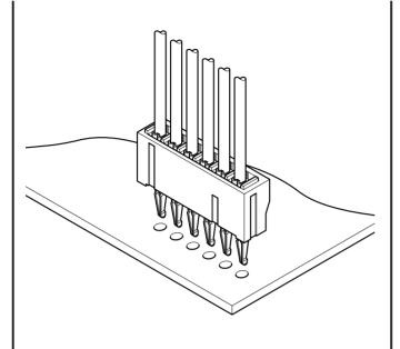
This low-profile, board-in connector, with a mounting height of only 4.25mm and a thickness of 2.4mm, is soldered directly onto printed circuit boards. The solder tail of the contact is resilient for easy assembly. The housing lances facilitate insertion of contacts.
