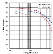
Model No: 10PM-K405B/K406B Driver: Chopper Dual Supply Voltage: 24.0 (Volt)
