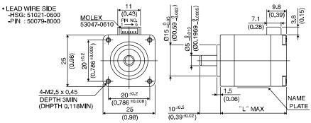
取付寸法 28mm タイプも御座います。 Motor frame size of 28mm is also available.
