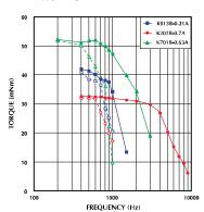
Model No: 10PM-K105B/K106B Driver: Chopper Dual Supply Voltage: 24.0 (Volt)
