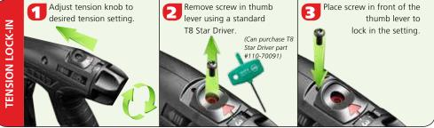
The EVO 9 quick-adjust tension feature allows for easy, blind tension adjustments; useful when using more than one cable tie type during an assembly application.
