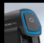
Visual warning: too cold = blue
