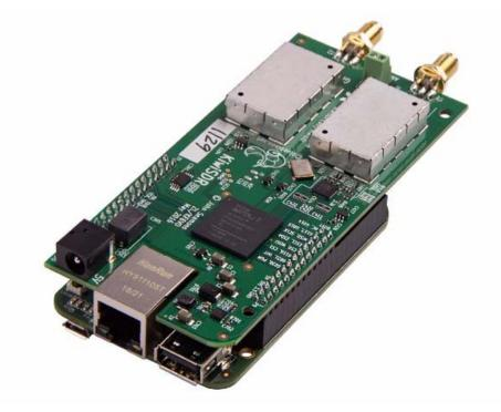
KiwiSDR is a software-defined radio (SDR) covering shortwave, the longwave & AM broadcast bands, various utility stations, and amateur radio transmissions, world-wide, in the spectrum from 10 kHz to 30 MHz.
