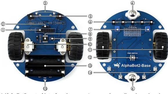
1. AlphaBot2 control interface: for connecting sorts of controller adapter board
