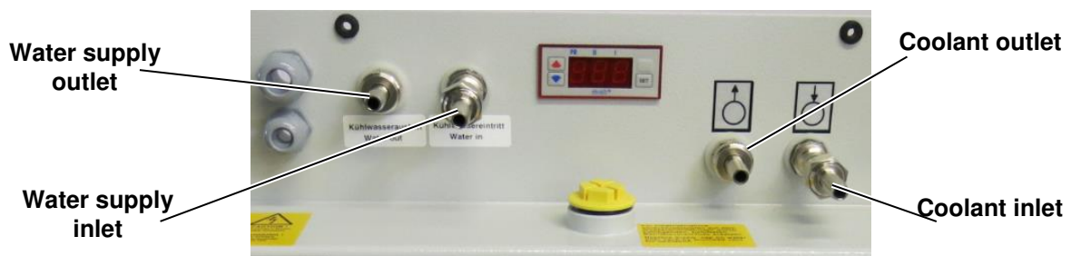
Fig. 8: Labelling of water inlet and water outlet
