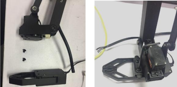
Step 2: Plug the wire of gripper
