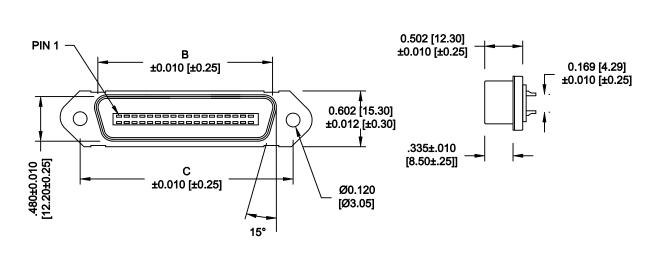
111-YYY-1 0 3 L 00 1 **SERIES POSITIONS** 014 024 036 050 GENDER 1 = MALE **TERMINATION** 0 = SOLDER CUP SHELL PLATING 3 = NICKEL **RoHS COMPLIANT-**L = LOW TEMP. PROCESS HARDWARE · 00 = NO HARDWARE PLATING 1 = GOLD FLASH
