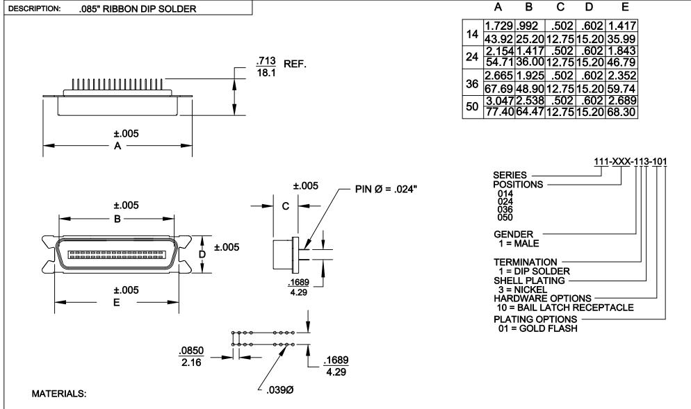
**INSULATOR: GLASS-FILLED THERMOPLASTIC UL RATED 94V-0 CONTACTS: COPPER ALLOY**
