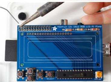
Now we will solder all 26 pins for the plate - this will send power and data between the two boards and also provide a mechanical stability. You may need to hold the plate down with tape to get it sitting flat against the Pi.
