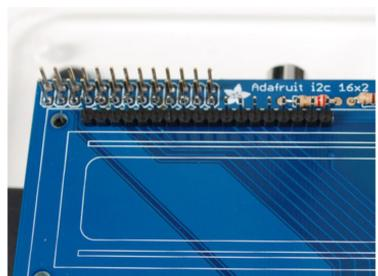
Finally, we place the LCD. Break off a piece of 18 or 16 pin header from the stick in the kit.
