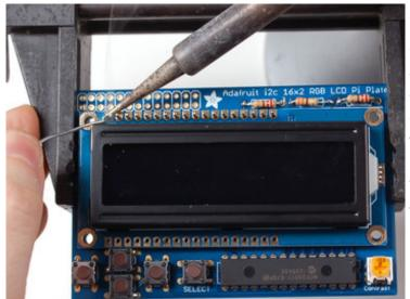
Your LCD may have two rows of connectors or one row. If its a two-row-connector LCD we do not use the bottom row, just continue using the LCD as it will fit just fine!
