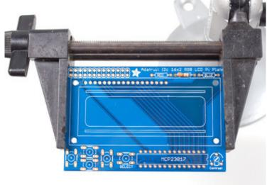
Put the printed circuit board into a vise or board holder, heat up your soldering iron and make sure you're ready to go!
