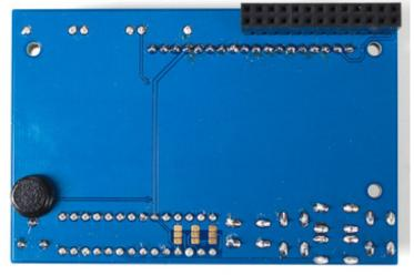
WARNING: If you're using the new Raspberry Pi model B+ with 4 USB ports you will need to take some extra steps to ensure the backlight resistor leads do not touch the USB ports and short out. See the steps below for more details.
