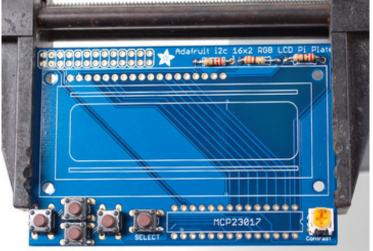
The kit may come with two potentiometers - a big blue one for breadboarding the LCD and a smaller orange one for the shield kit. You can throw away or recycle the blue one, use only the orange one here!
