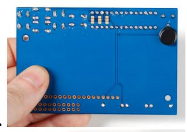
On kits where the buttons are on the left, put it right below the contrast pot, as shown. This will keep the pot from touching the Ethernet jack.
