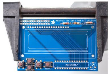
up/down/left/right input and a button to the right called SELECT. These 5 buttons should be able to make 'talking' back to your project easy. These are connected to the I2C port expander chip so they require no extra pins on the Pi, our library does the work of reading whether they are pressed.
