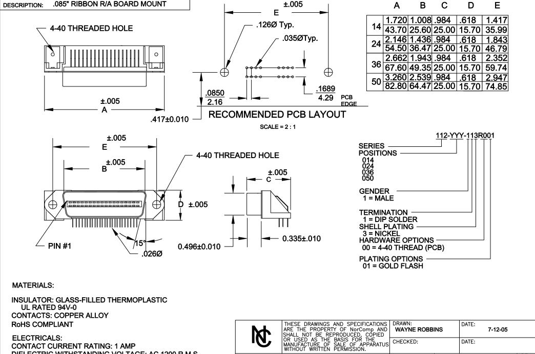
**ELECTRICALS: CONTACT CURRENT RATING: 1 AMP** DIELECTRIC WITHSTANDING VOLTAGE: AC 1200 R.M.S. INSULATION RESISTANCE: 1000 mohms MINIMUM AT 500V DC **CONTACT RESISTANCE: 30 mOHMS MAXIMUM**
