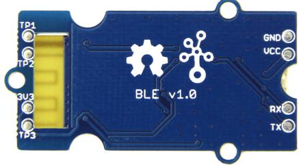
Grove - BLE v1 (Grove - Bluetooth Low Energy v1) uses a Low Energy Bluetooth module -- **HM-11**, based on TI CC2540 chip, which has AT command support. As a Grove product it's convenient to use Grove - BLE with Arduino board via Base Shield.
