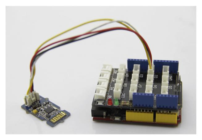
Grove - BLE can be used as a master or slave, you can use the one via different demos. If you are going to use the following SoftwareSerial program, please refer to the way of connection in the previous pic.  $TX \rightarrow D2$ ,  $RX \rightarrow D3$ .
