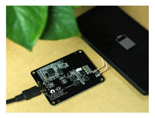
Your phone will enter the charging mode when D1 is flashing and buzzer is turned on.
