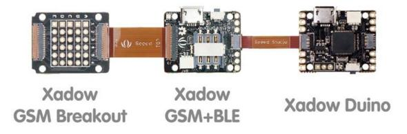
RePhone Lumi Kit is specially designed for LED lovers - embedding the Xadow GSM+BLE module into your awesome lighting device and control the light via SMS or Bluetooth!
