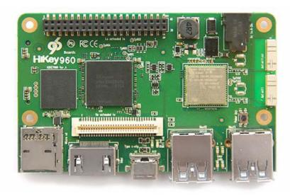
The HiKey 960 is powered by the latest Kirin 960 SoC with four ARM Cortex-A73 CPUs (up to 2.3GHz) and four ARM Cortex-A53 CPUs (up to 1.8GHz) configured according to the big.LITTLE architecture. The integrated Mali<sup>TM</sup>-G71 MP8 GPU in the Kirin 960 SoC gives the HiKey 960 high performance image processing abilities. With 3GB LPDDR4 memory and 32GB UFS flash on board, the HiKey 960 can be used for most embedded applications.
