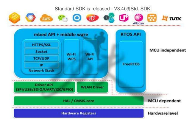
Full-fledged Standard SDK is now released for download. In the Standard SDK, we provide support to cost-effective Ameba IC and connect to a number of cloud services easily. With the detailed control in all aspects, Standard SDK is your best choice. Please refer to Getting Started.
