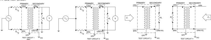
Measurement instruments: Hp4192a Impedance Analyzer; Hp3456a DVM; Keithley 2002 DVM; D scope series iii audio analyzer
