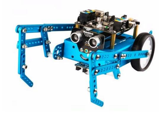
mBot six-legged robot is a 3-in-1 expansion pack based on mBot.
