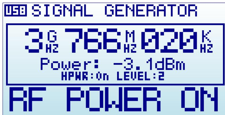
Please note standard precaution of RF power delivered without a connected load.
