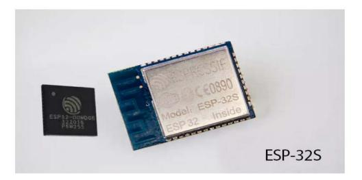
ESP-32S Wifi Bluetooth combo module is ultra high performance and ultra low-power consumption Wi-Fi and Bluetooth combo wireless platform based on ESPRESSIF ESP32 chipset. ESP-32S integrates dual-core processor, 448 KByte ROM,520 KByte SRAM,16 KByte SRAM in RTC, 802.11 b/g/n/e/l Wi-Fi, Bluetooth v4.2 BR/EDR & BLE, clocks & Times, abundant peripheral Interfaces and sercurity mechanism.
