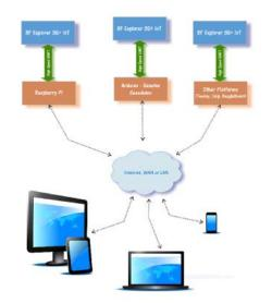
Furthermore, other platforms such as BeagleBone, Chip, Chipkit, Teensy all them can easily control a RF Explorer 3G+ IoT by manually connecting to a standard UART port.
