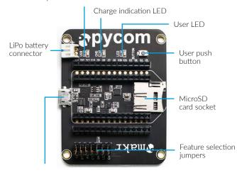
Micro USB connector for power and serieal communication
