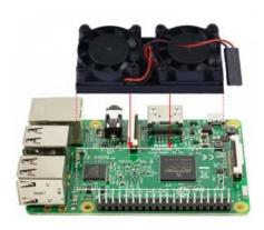
Is your RaspberryPi overheating? Whether it's in a hot environment or your RPi is crunching non-stop we have a solution – the Raspberry Pi Ultimate Cooling Dual Fan!
