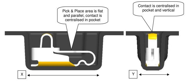
2) Possible out of position situation for the contact in the pocket. This can not be controlled or avoided but it can be dealt with during pick and place to enable the contact to be pick and place. The component will usually vibrate down into the pocket once the cover tape is removed and the feeder indexes. Providing the correct nozzle type is used and the correct offset position, the nozzle can be used to nudge the contact down into the pocket
