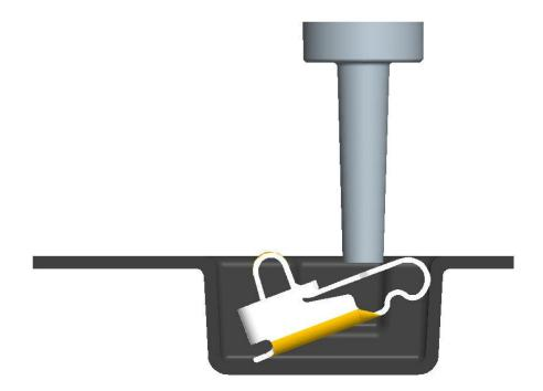
Once the cover tape is removed from the pocket, if the vibration and shock of the feeding mechanism on the machine is too violent, the contacts could jump out of position in the tape, or even jump out of the pocket due to their low mass.
